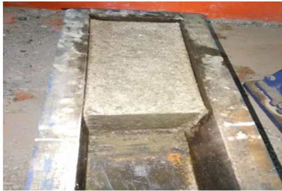
Fig. 3 Bricks prepared from shredded plastic with cement and fly ash
