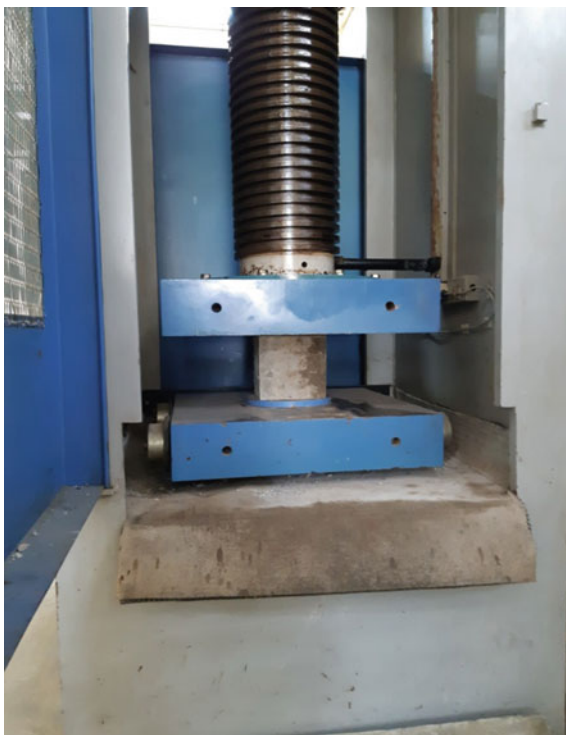
Fig. 3 Testing of cube specimens (before the start of test)
