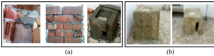
Fig. 7 Small-scale model house. a Conventional using bricks and concrete; b mud composite
