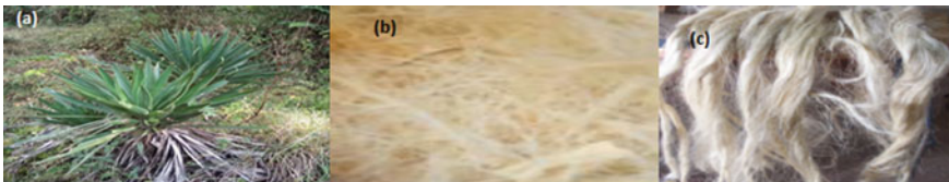
Fig. 1 Sisal fiber a Sisal plant, b Processed sisal fiber and c Sisal fiber image, according to Uppal et al. [10]
