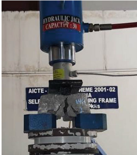
Fig. 3 Edge notched disc bend (ENDB) specimen against Mode-I fracture test setup
