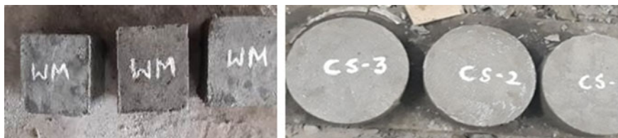
Fig. 2 Concrete cubes and cylindrical specimens against compressive strength test
