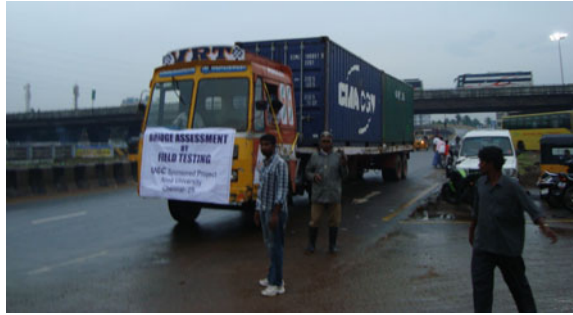
Fig. 7 Truck employed for bridge testing
