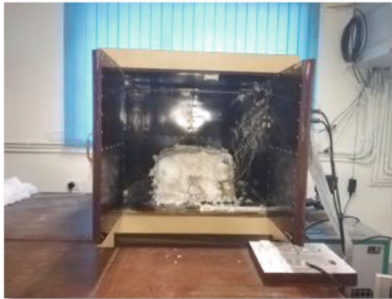
Fig. 8 Thermal conductivity test set up
