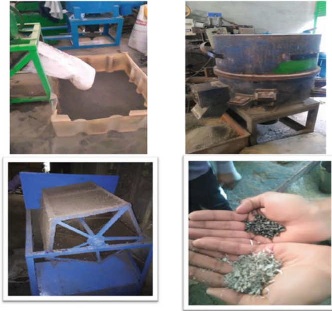
Fig. 2 Shredded plastic in powdered (aggl) form with sieve and grinder
