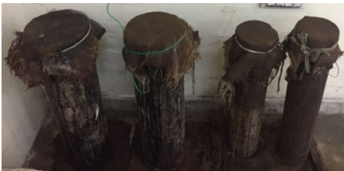
Fig. 3 Wet burlap used to close the CFST specimens
