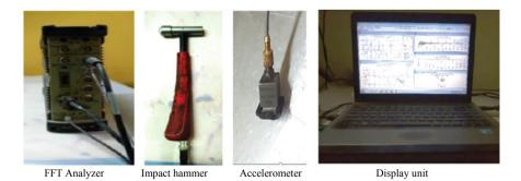
Fig. 6 The test set up for vibration measurement
