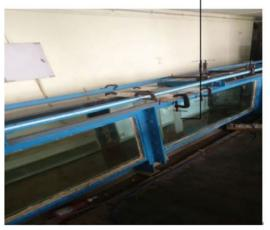
part represents the reservoir, in which water is filled up to certain different heights, and the inflow was then stopped. The water supply system comprises a constant head reservoir (dam reservoir) at an elevation of about 2 m above the ground level. Pumps are used to lift water from the underground reservoir to the dam reservoir. The constant discharge was maintained to minimize the waves formed in the storage behind the dam.
