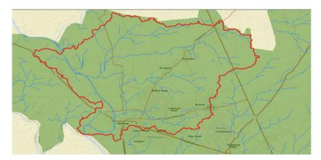
Fig. 2 Delineated basin using flow accumulation
