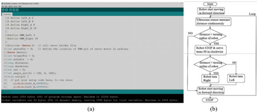
Fig. 21.4 a A program in Arduino IDE software. b A detailed flowchart of a program
