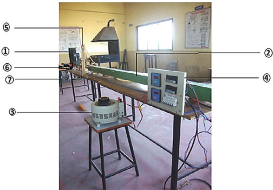
Fig. 54.1 Experimental setup (1 air blower, 2 square duct test section with casing, 3 dimmer start, 4 control panel, 5 U-tube differential vertical manometer, 6 variable flows drive, 7 orifice setup and setting chamber)
