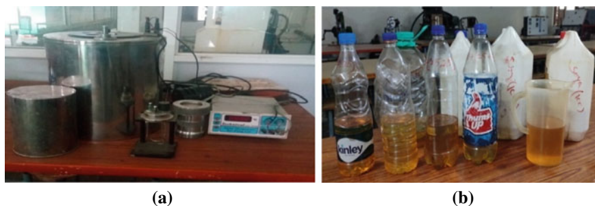
Fig. 37.2 a Bomb calorimeter and b prepared biodiesel samples
