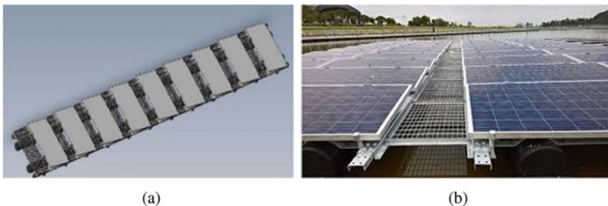
Fig. 13.3 a Polyethylene rafts supporting 9 PV modules, b raft with catwalks [17, 19, 20]
