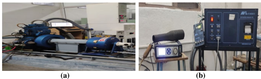
Fig. 37.1 a Engine setup and b smoke meter and gas analyzer
