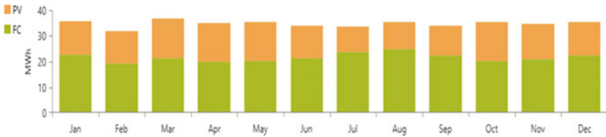
Fig. 26.4 Monthly electric production by solar PV-fuel cell-battery
