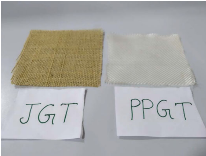
Fig. 1 Photographic view of woven jute geotextile and polypropylene geotextile
