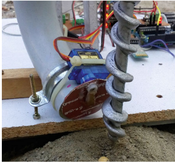
Fig. 6 Servomotor controlled lid and drill bit
