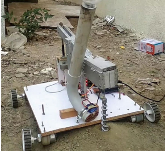
Fig. 9 Prototype model of seed sowing robot
