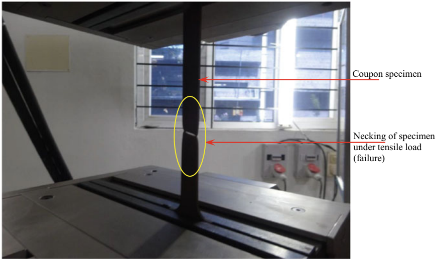
Fig. 4 Failure of a coupon under tensile load
