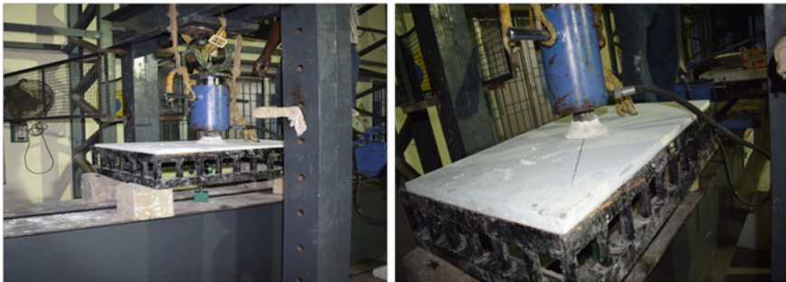
Fig. 5 Slabs under deflection load
