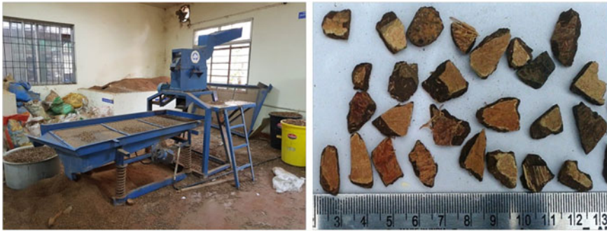
Fig. 1 a Coconut shell crusher, b Crushed coconut shells
