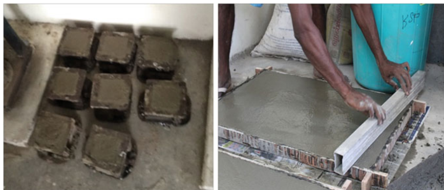
Fig. 2 Sample of cast specimens a cube b slab
