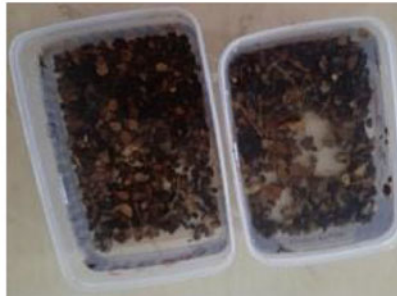
(f) Water absorption test: RCS(T2W) & ODCS(T2W)
