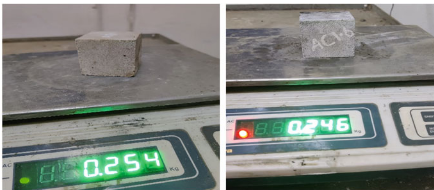
Fig. 4 The sample density observation value of aquatic CaCO 3 mortar
