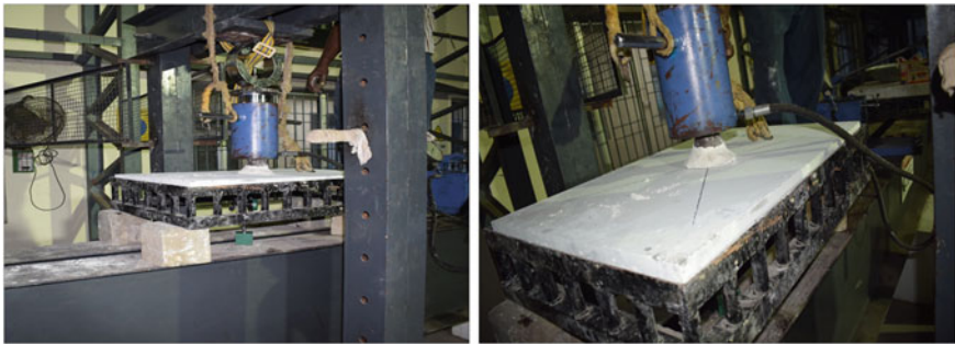
Fig. 5 Slabs under deflection load
