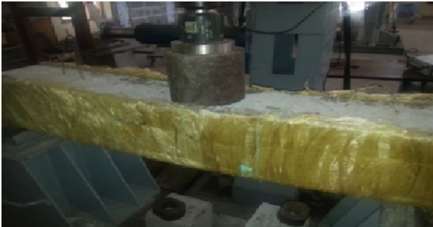
Fig. 8 Typical view of testing of wrapping of sisal fibre RCC beam
