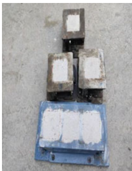
Fig. 8 The casting of cube for 30% of aerogel
