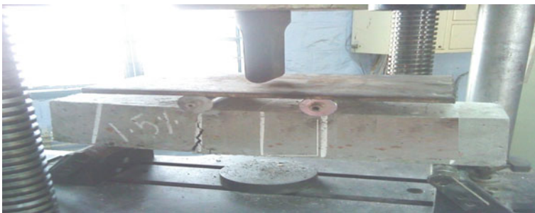
Fig. 8 Modulus of rupture test—prism specimen
