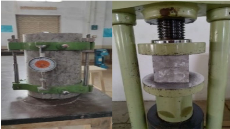
Fig. 1 Compression test for cubes and cylinders sample
