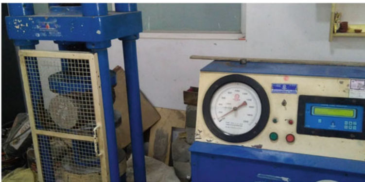
Fig. 6 Split tensile strength test on cylinder
