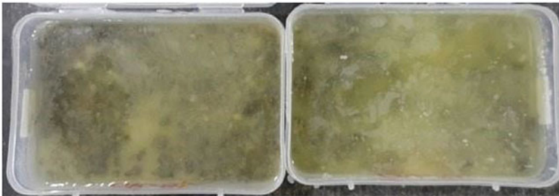
(e) Water absorption test: RCS(T1W) & ODCS(T1W)
