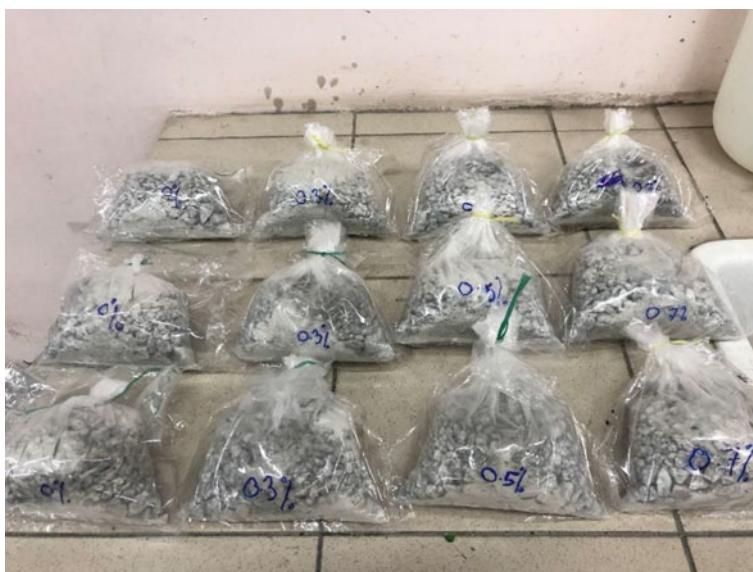
Fig. 2 Aggregate preparation for Marshall mix
