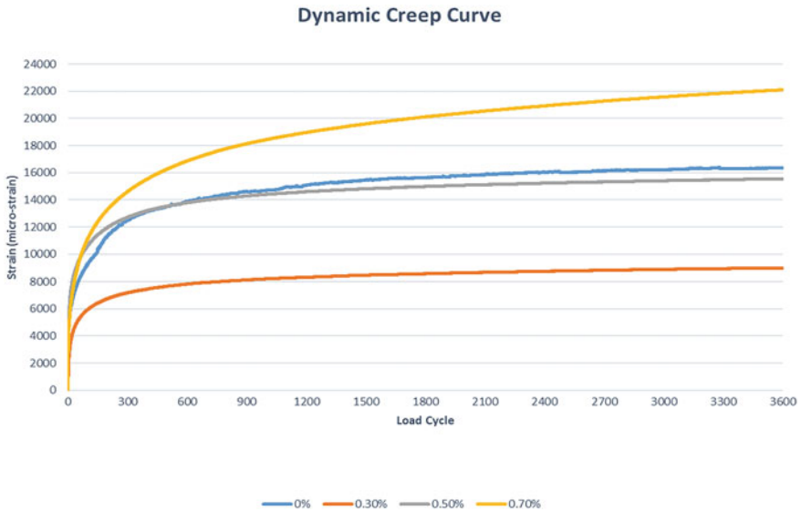
Fig. 11 Dynamic creep curve of SMA mixture
