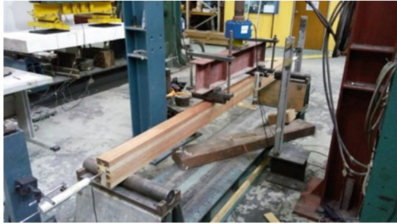
Fig. 6 Test sample laid out ready for the flexural test with LVDT mounted at each end and in the middle of the beam span
