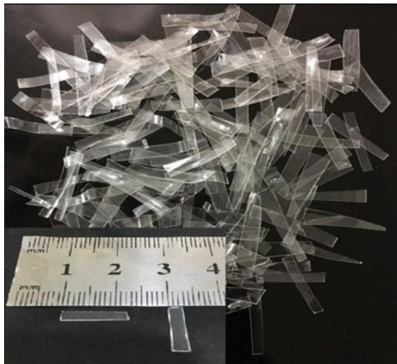
Fig. 3 Recycled PET use as fibre (Alfahdawi et al. 2019)
