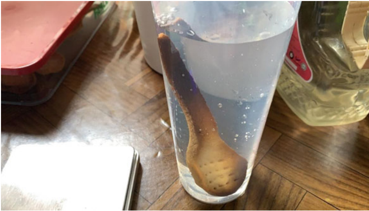
Fig. 3 Water absorption test for edible cutleries
