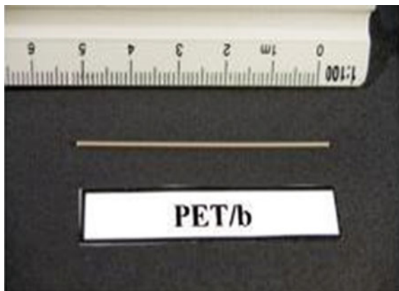
Fig. 7 Straight fibre shape (Fraternali et al. 2011)
