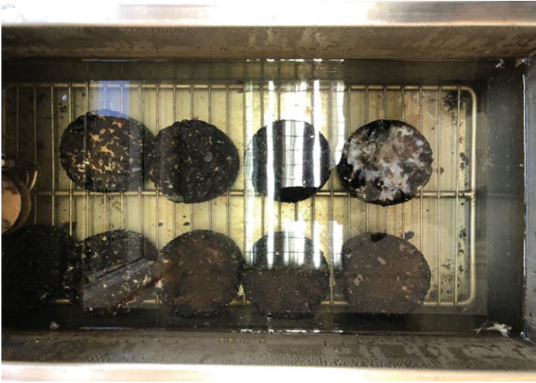
Fig. 3 All samples immersed in the 60 °C water bath
