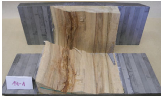
Fig. 8 Rolling shear failure of beech lamination (Source Aicher et al. 2016)
