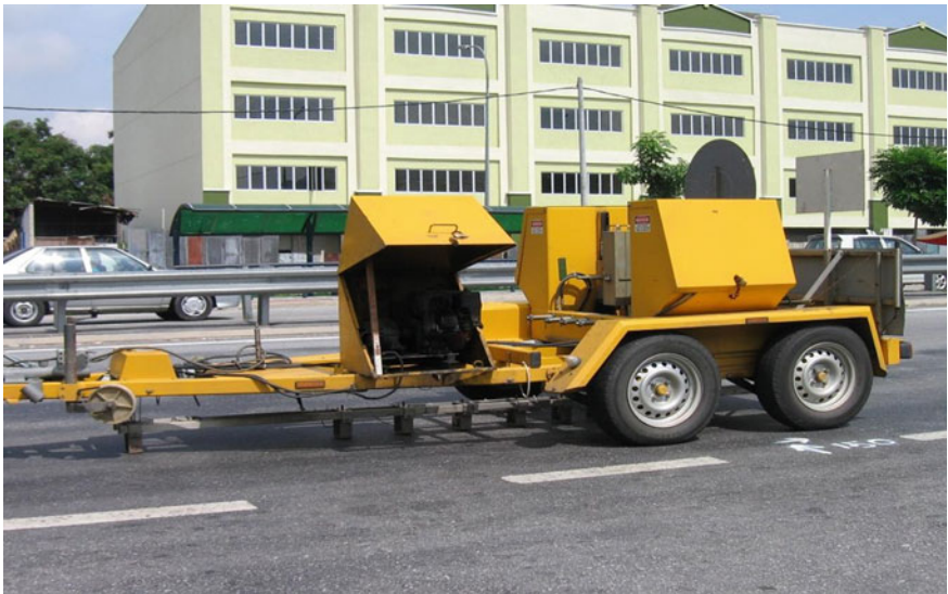
Fig. 10 Falling weight deflectometer
