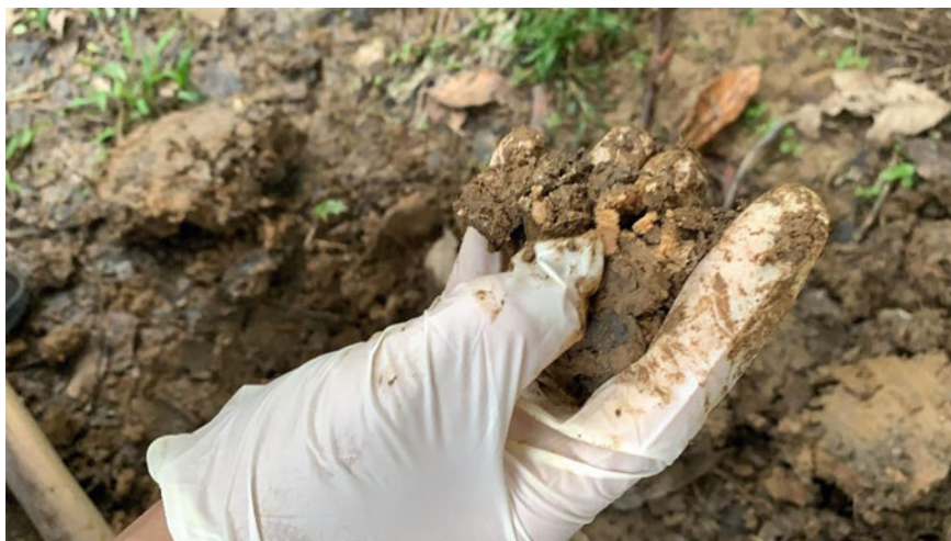
Fig. 8 Edible cutleries after 3 days of soil burial test
