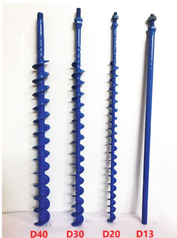
Fig. 1 Model piles used in tests
