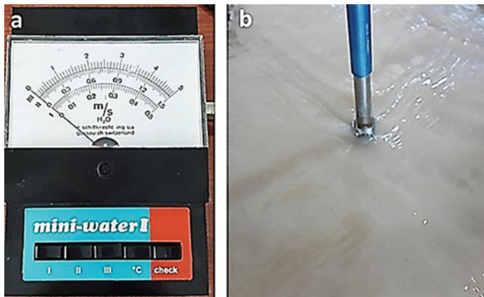
Fig. 8 Flowmeter device; a control panel box, b small fan
