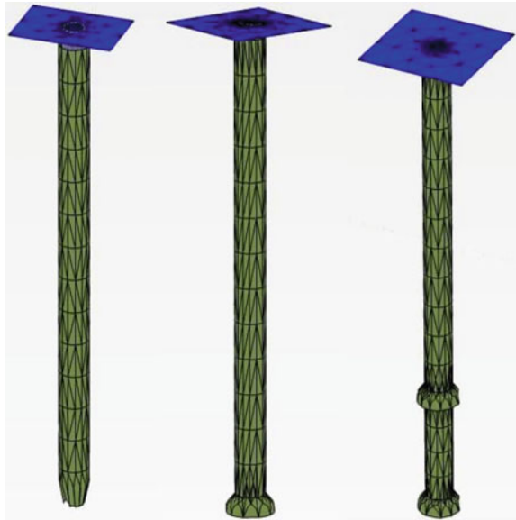
Fig. 8 Finite element mesh of pile
