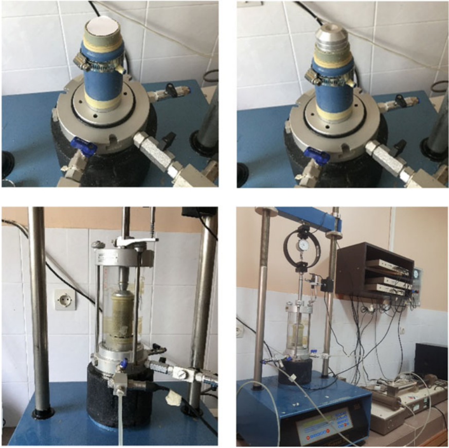
Fig. 4 The triaxial cell and was assembled and filled with water
