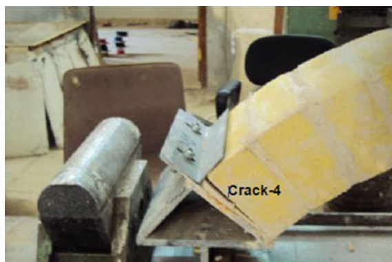
Fig. 10 Crack 4 occurred at the nearest end
