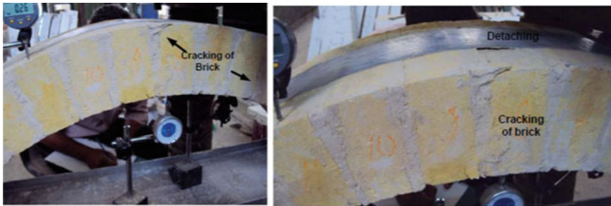
Fig. 16 Cracking of bricks and mortar, and starting of detaching
