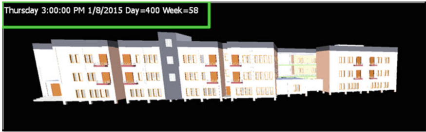
Fig. 10 Video screenshot for planned project progress at 400 days
