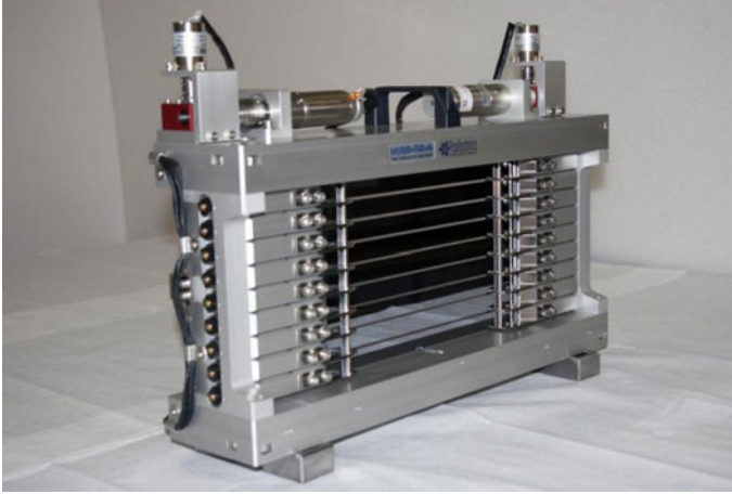
Fig. 3.11 Multiple single crystal based neutron monochromator (reproduced with permission from Mirrortron Ltd.)
