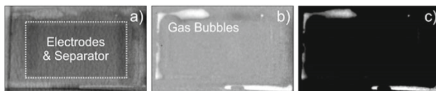
Fig. 10.11 Neutron transmission images of a pouch cell illustrating the different processing steps. a After noise reduction, b after normalization to the first image and c after segmentation, with grey areas representing the generated gas [16] (open access)
