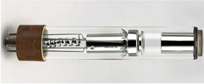
Fig. 2.9 Photograph of very compact pulsed neutron tube used in IGN-1 and IGN-1-M developed by USSR
