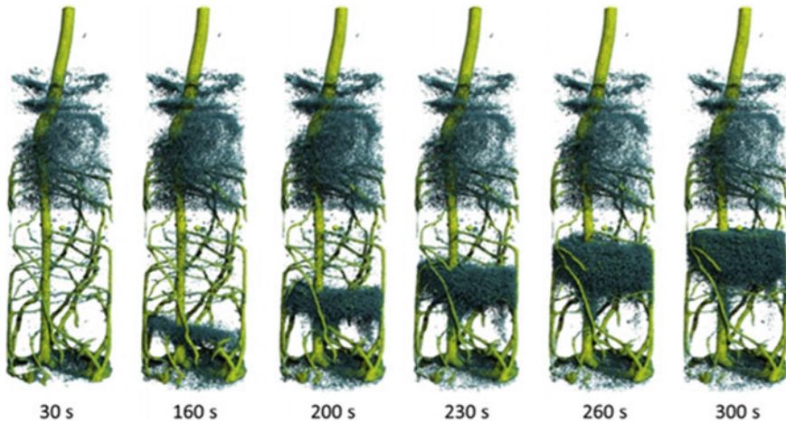
Fig. 11.6 Time-resolved neutron tomography of the root system of a lupine after injection of deuterated water through the bottom. From the tomographies conducted at different instants the movement of waterfront can be visualized [46] (Open access)
