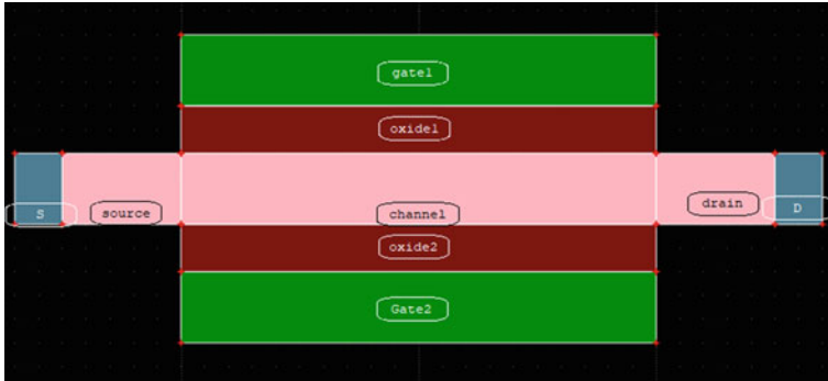
Fig. 1 Structure of Si-based DGMOSFET
