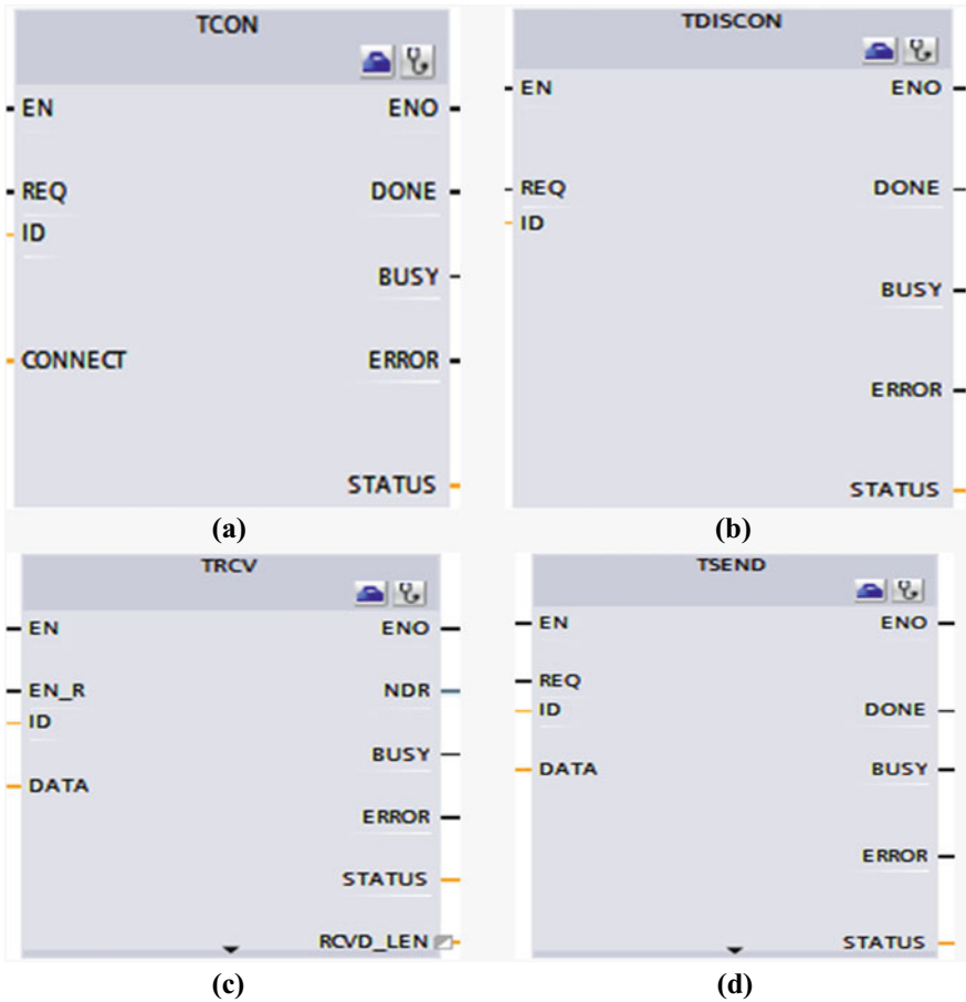
Fig. 9 a TCP connection start in TIA portal b TCP connection close in TIA portal c TCP receive in TIA portal d TCP send in TIA portal
