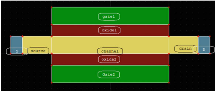
Fig. 2 Structure of Ge-based DG MOSFET
