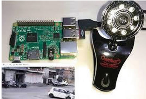
Fig. 12 Webcam connected via Raspberry Pi at location 2
