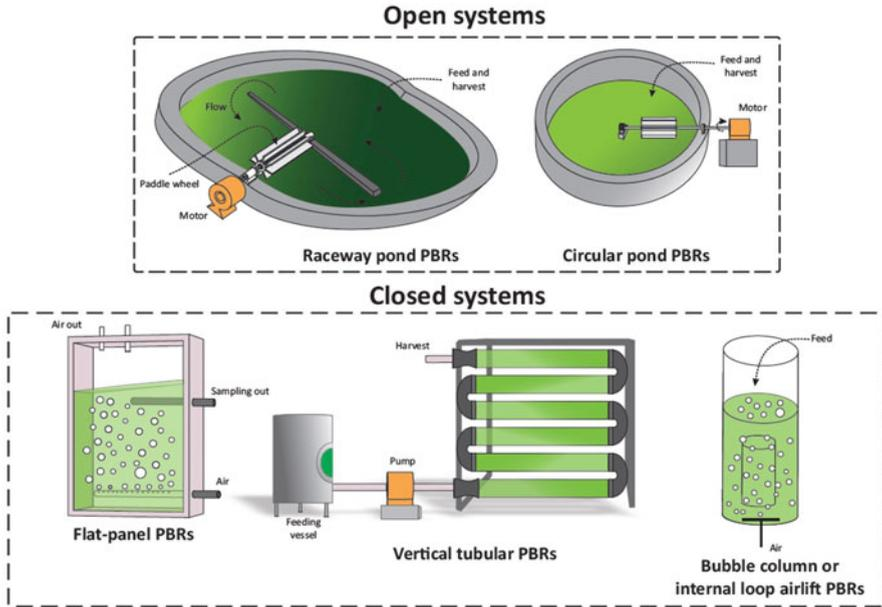
Fig. 12.2 Photobioreactors (PBRs) technology used for microalgae culture
