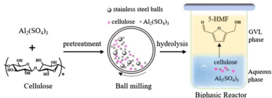
Fig. 10.3 \text{Al}_2(\text{SO}_4)_3 -assisted mechanochemical synthesis of 5-HMF from cellulose (Reprinted with permission from [36]. Copyright ©2020, Springer)
