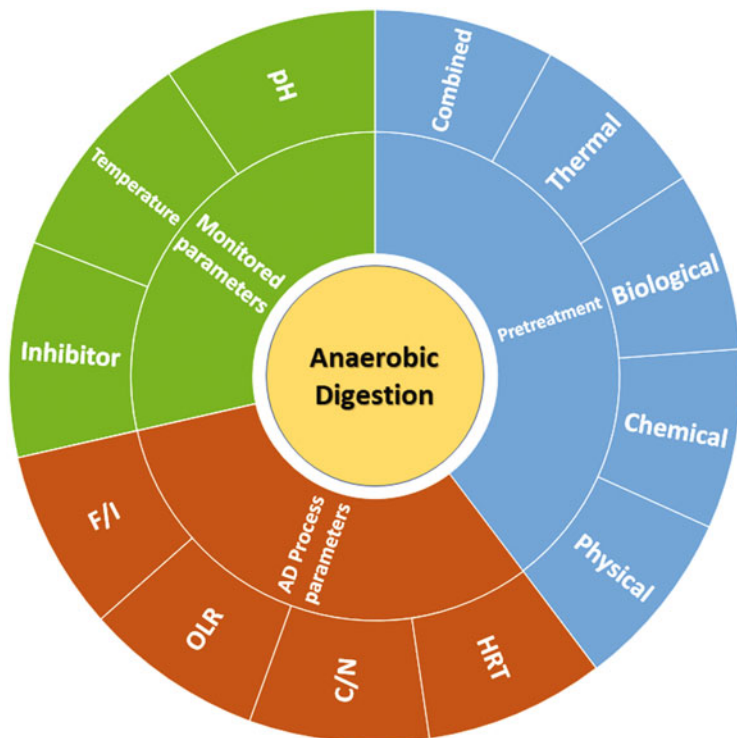
Fig. 6.3 Summary of the various process parameters, parameters to be monitored, and pretreatment techniques. In orange are the AD process parameters: Feed/inoculum ratio (F/I); organic loading rate (OLR), carbon/nitrogen ratio (C/N) in the feed, and hydraulic retention time (HRT). In brown are the parameters needed to be monitored during the AD of SOWs (pH, temperature, and inhibitors). In green are the different pretreatment methods used to improve AD yield
