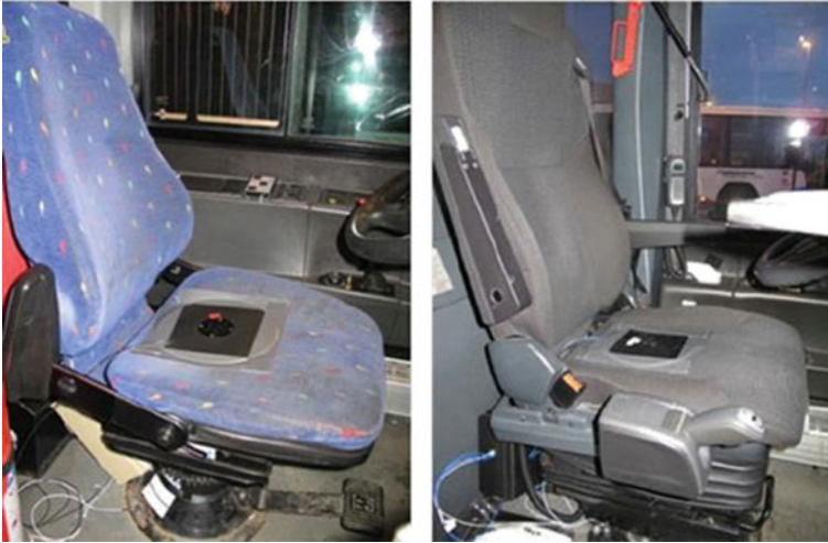
Fig. 13.9 The pedestal seat (left) and air-suspension seat (right) used in the study (Jonsson et al. 2014)
