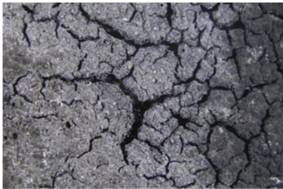
Fig. 8.10 Digital photograph of the residue of PA 6/organoclay (90/10) nanocomposites after combustion test (Dasari et al. 2007)
