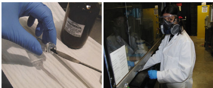
Fig. 7.15 Protection methods for handling potentially hazardous engineered nanomaterials in laboratory conditions (Haynes and Asmatulu 2013)
