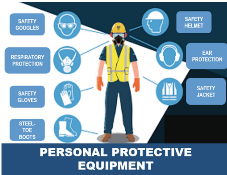
Fig. 4.1 Personal protective equipment to protect the operator from hazards (Loibner et al. 2019)
