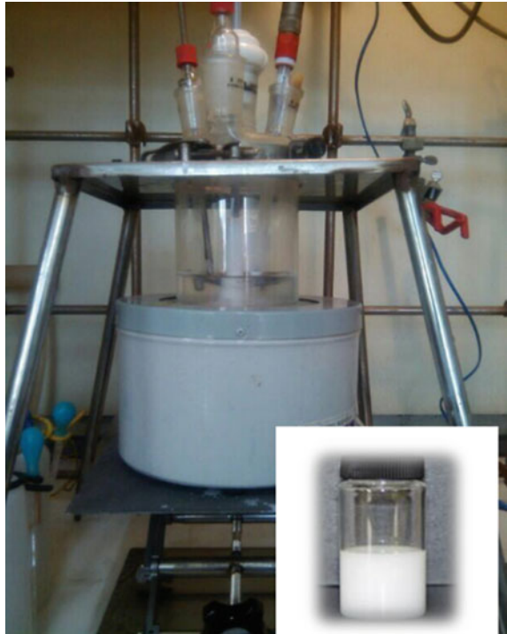
Fig. 3.5 UF resin synthesis and its results in the laboratory (Nuryawan et al. 2017)
