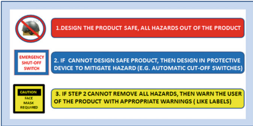
Fig. 5.1 Three vital aspects of design for safety
