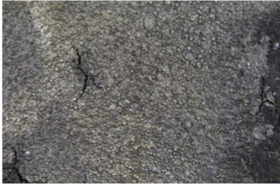
Fig. 8.11 Digital photograph of the residue of PA 6/organoclay (70/30) nanocomposites after combustion test (Dasari et al. 2007)
