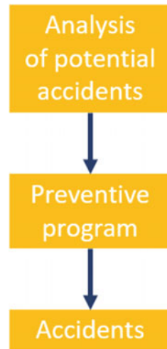
Fig. 1.1 Reactive approach for deriving preventive actions from accidents (Brauer 2005)
