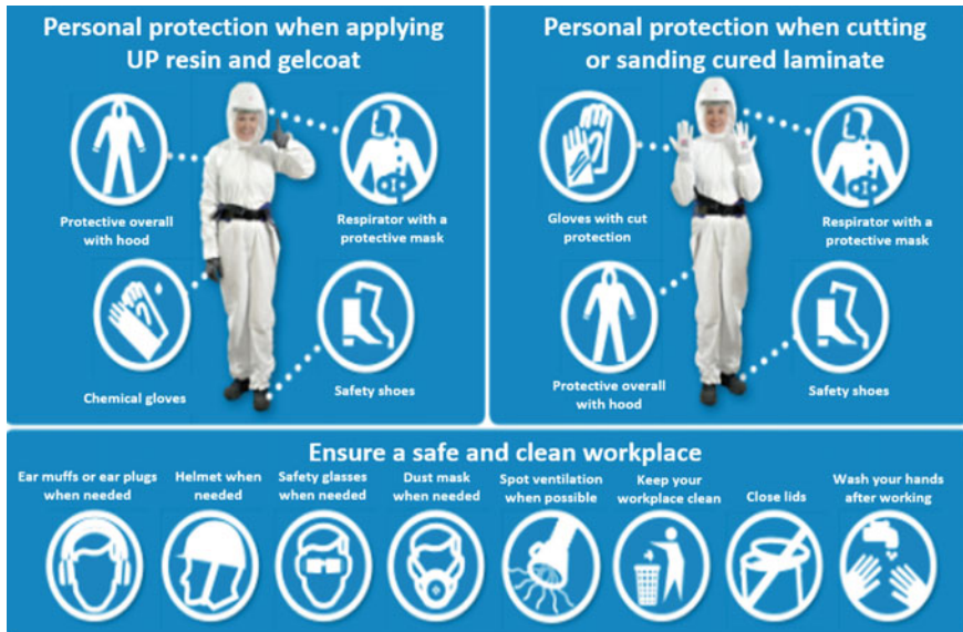
Fig. 7.14 Safe handling guides (The European UP/VE Resin Association 2018)
