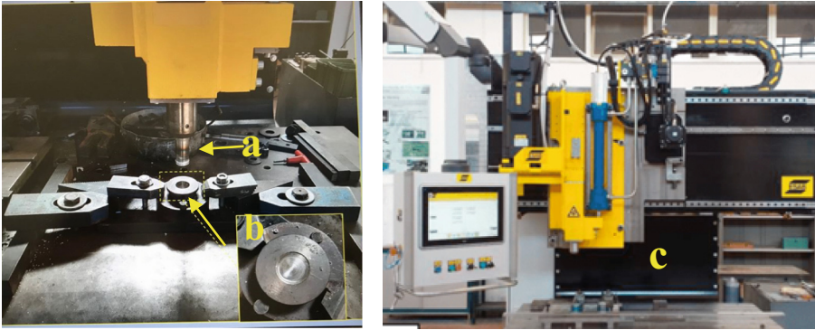
Fig. 1. (a) Tool, (b) die & (c) ESAB LEGIO
