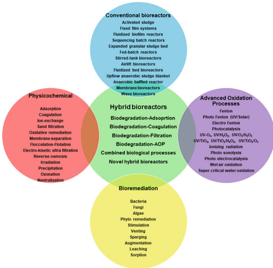
Fig. 1 Broad spectrum of combinations in treatment of dye effluents by hybrid bioreactors
