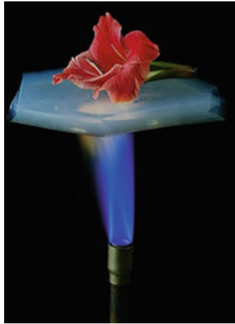
Fig. 3 A silica aerogel slab protecting a delicate flower from excessive heat generated from a burner ( https://commons.wikimedia.org/wiki/File:Aerogelflower_filtered.jpg )
