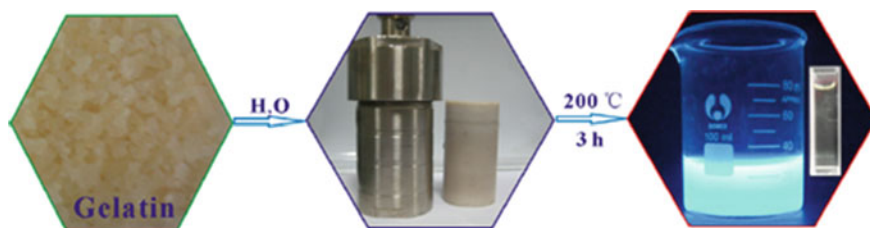
Fig. 2 Graphical abstract of the photoluminescent carbon dots synthesis based on commercial gelatine using a hydrothermal treatment. (By Liang et al. [40], License number 4960230818190 provided by Elsevier and Copyright Clearance Center)
