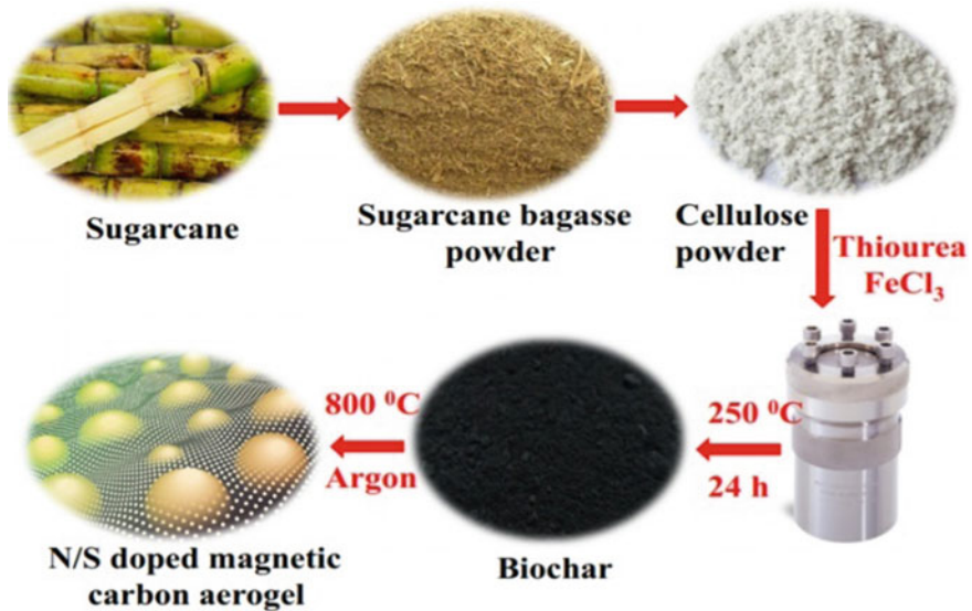
Fig. 18 Preparation of N/S-doped magnetic aerogel from sugarcane bagasse [5]
