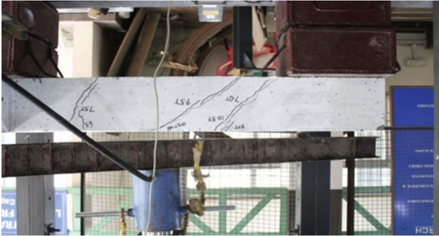
Fig. 7 Specimen during testing (Spiral Crack)
