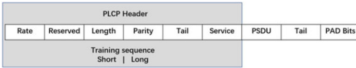
Fig. 4.8 IEEE 802.11p PPDU architecture
