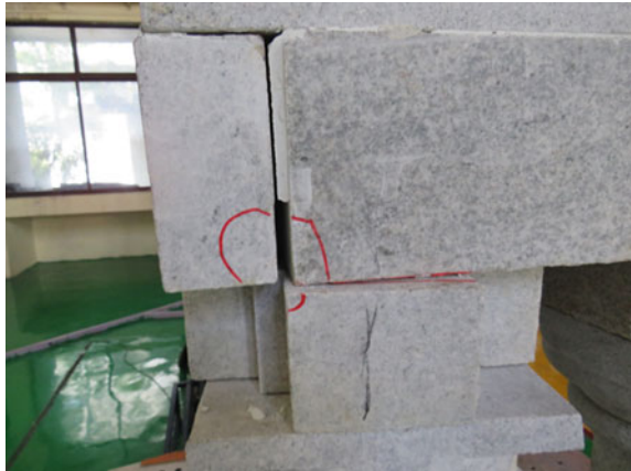
Fig. 13 Displacement of the beams
