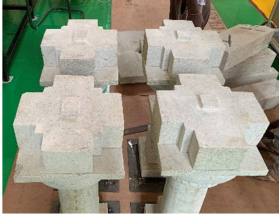
Fig. 7 Table joints provided in the model for various elements of the column
