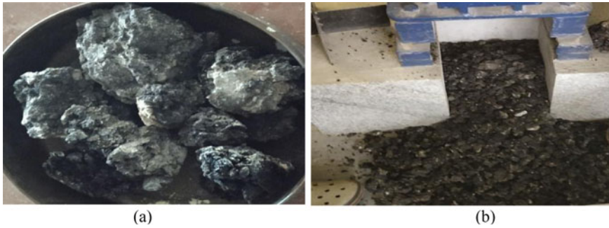
Fig. 4 RAP a in its original form and b after processing through jaw crusher
