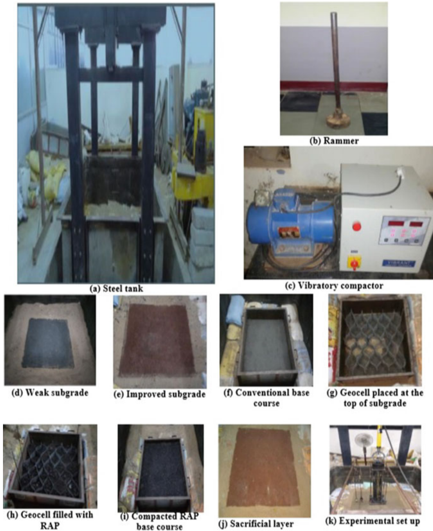
Fig. 6 Schematic representation of stage construction adopted during the construction of model pavement sections and experimental set up.
