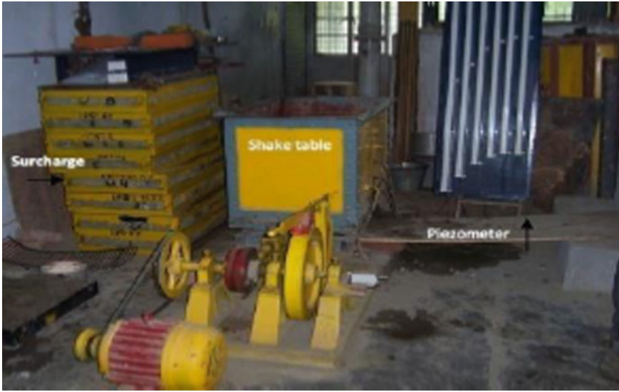
Fig. 3 View of shake table, surcharge weights, and piezometers
