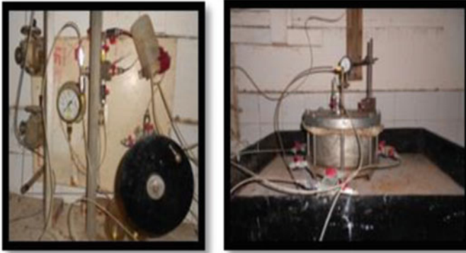
Fig. 3 Rowe Type oedometer and self-compensating mercury
