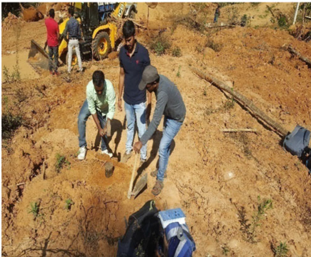
Fig.3 Collection of soil samples at landslide affected area
