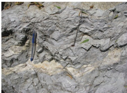
B) Dol. Lst. with numerous closely spaced joints and ~5 cm thick calcite vein
