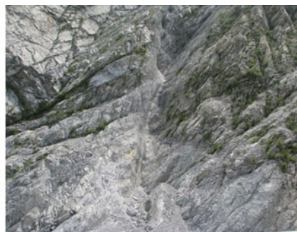
D) Shear/fault zone with gouge in the center. Thickness of gouge is 15 cm
