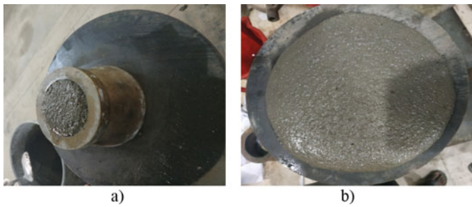
Fig. 1 a Mortar sample in brass mold and b Sample shape turned into a pancake shape
