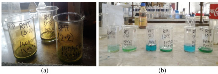
Fig. 3 Experimental process. a Brown NO 2 gas formed at stage 2. b Final solution for analysis
