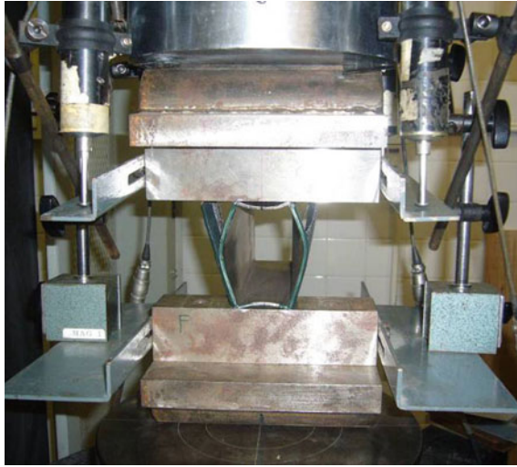
Fig. 8 Failure mode in ETF condition
