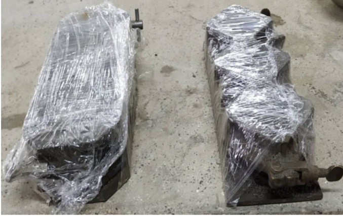
Fig. 4 Wrapped finished sample inside the molds before heat curing
