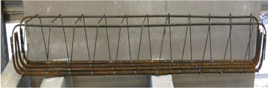
Fig. 1 Beam with continuous spiral reinforcement
