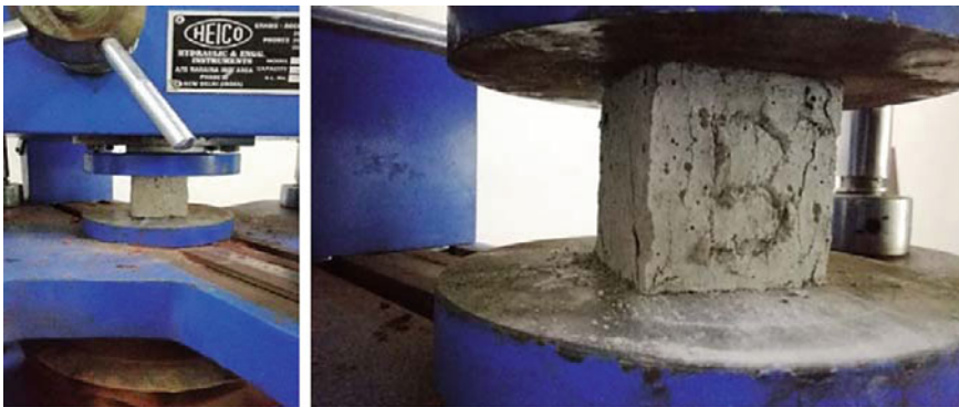
Fig. 3 Compressive strength of cubes at 28 days
