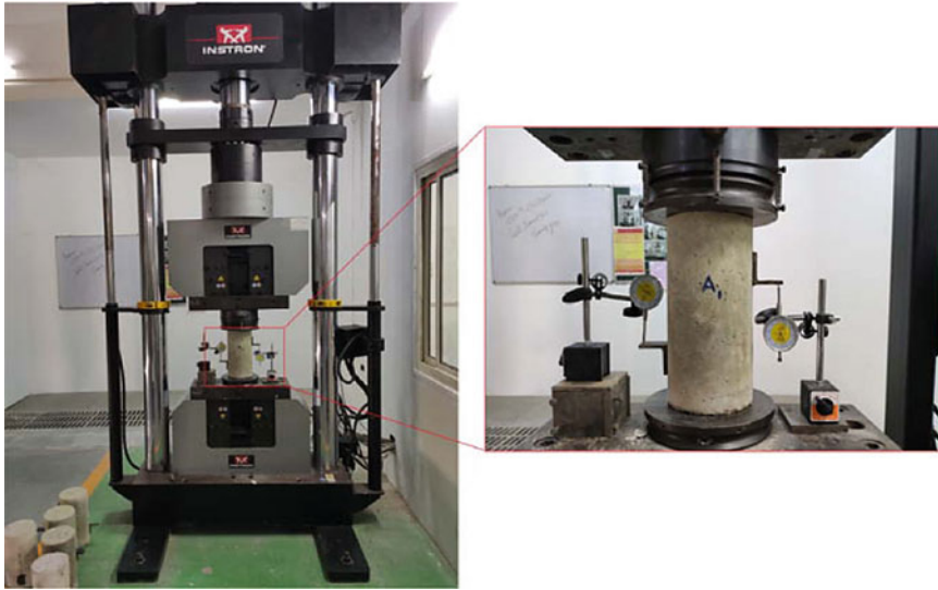
Fig. 4 Set-up of cylinder specimen A under UTM
