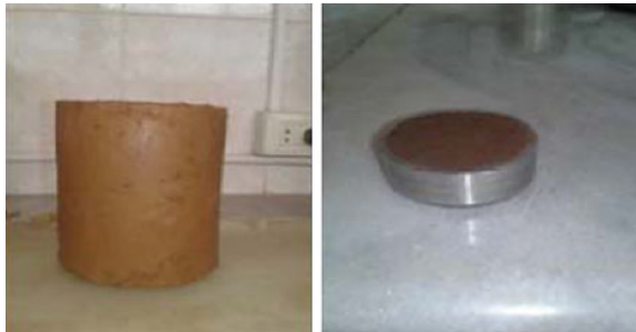
Fig. 2 Remolded samples in laboratory (Proctor sample, Oedometer sample)
