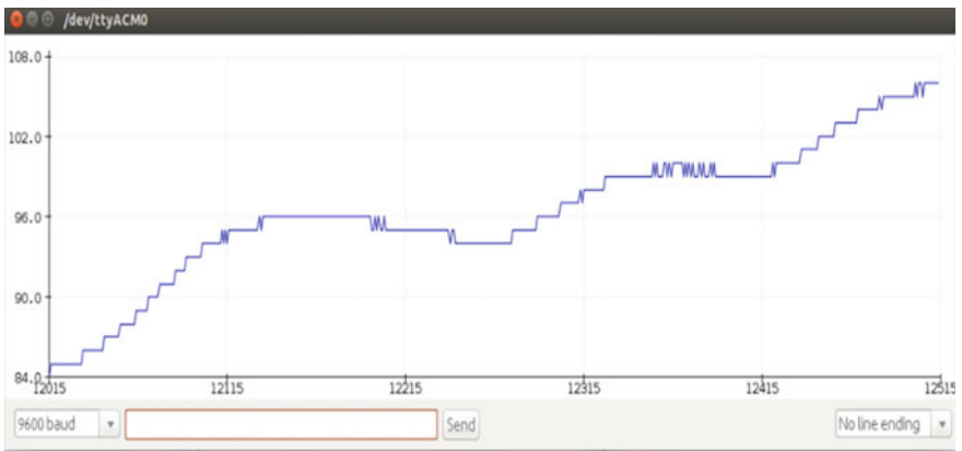
Fig. 10 Serial monitor graph when the gas detection is present (x-axis = time, y-axis = ppm)
