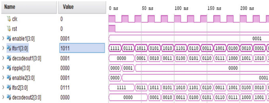
Fig. 6 Simulation result of multistage LFSR counter using methodology proposed in [4]
