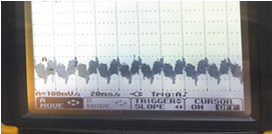
Fig. 12 Performance of the jammer device as a simulated waveform (FLUKE Device)
