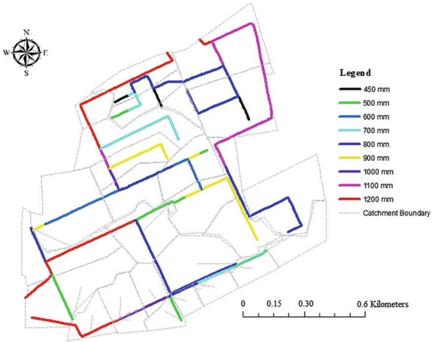
Fig. 6 Layout of Pipe network for stormwater drainage
