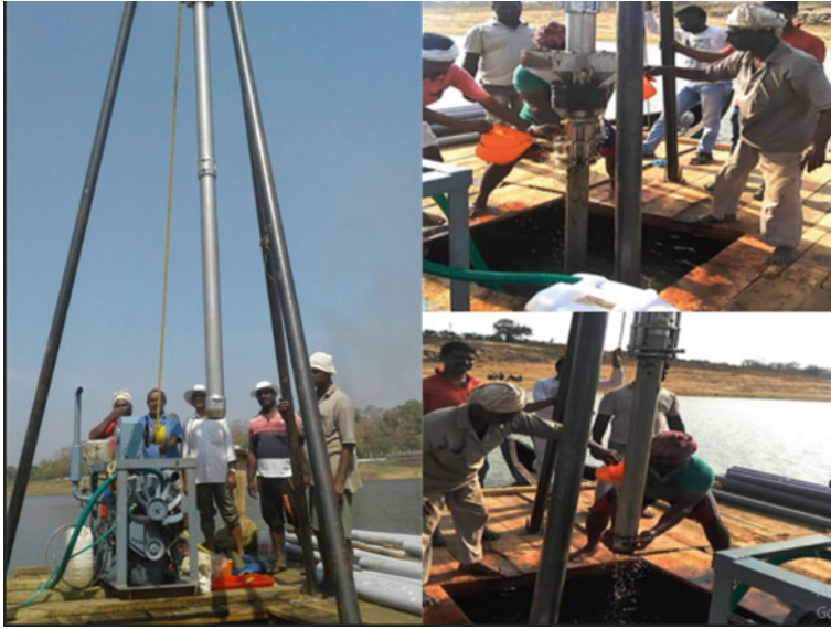
Fig. 3 Sample Collection using Gravity Corer
