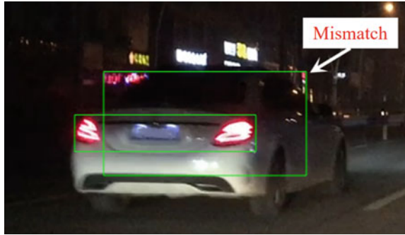
Fig. 21 Mismatch of interference light source1.25
