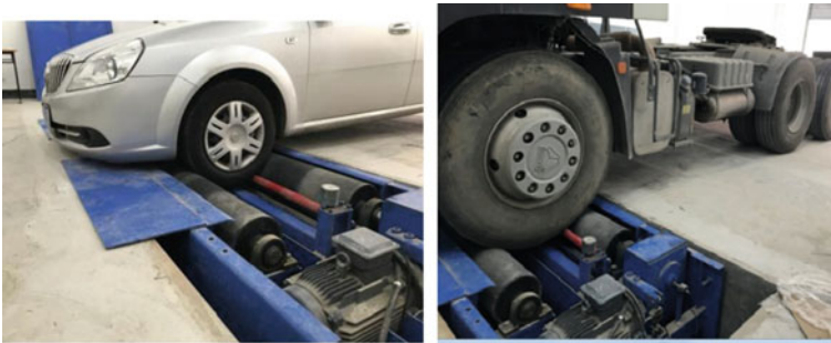
Fig. 2 The experiment of the influence of different roller center distances on the detection of braking force
