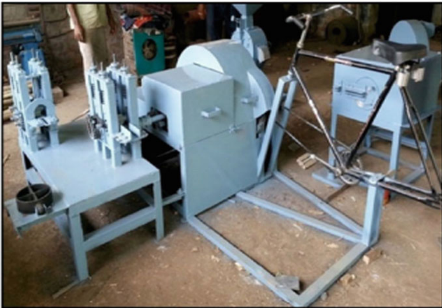
Fig. 9 Bamboo slivering operated by HPFM [26]
