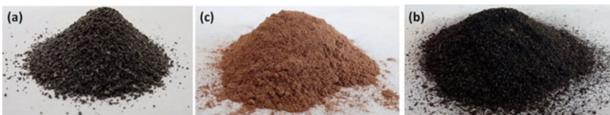
Fig. 1 Physical appearance of a stone dust, b bentonite clay, and c coal dust
