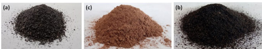
Fig. 1 Physical appearance of a slag, b bentonite clay and c coal dust
