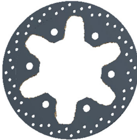
Fig. 9 Optimized geometry by topology optimization
