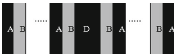
Fig. 1 Schematic diagram of 1-D photonic crystal with defect
