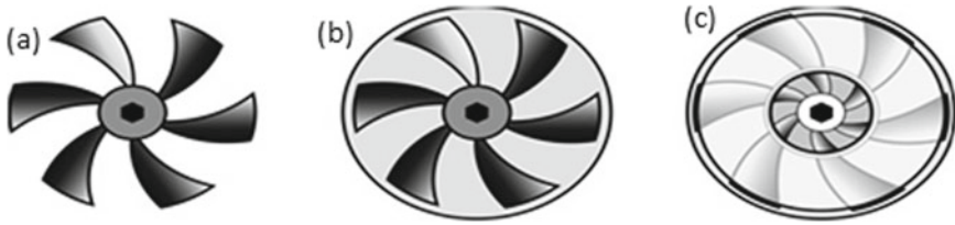
Fig. 1 Centrifugal impeller types a open; b semi-enclosed or semi-open; c enclosed
