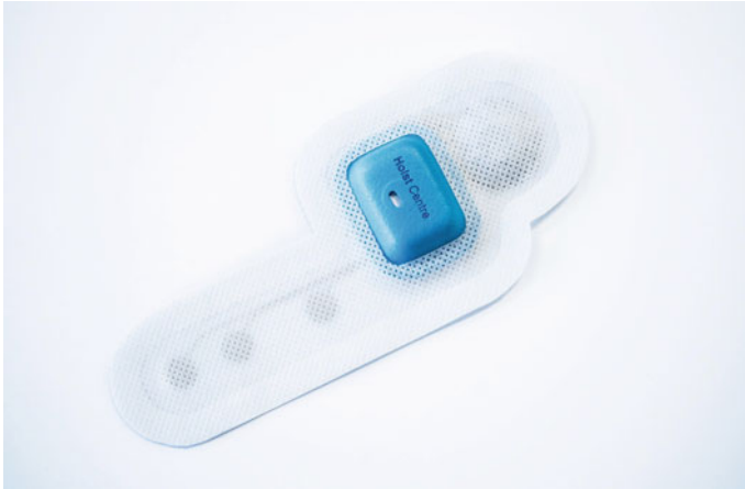
Fig. 8.3 Example of ECG chest patch
