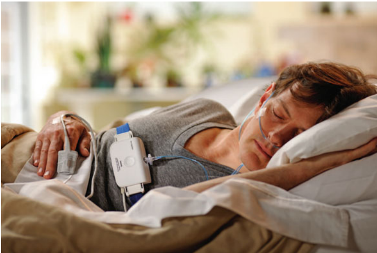
Fig. 8.2 Example of portable PG OOC device for home sleep monitoring. Courtesy of Philips Respironics, all rights reserved
