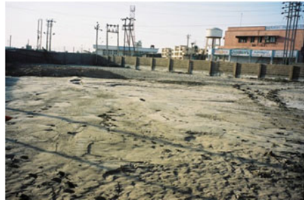
a Settlement of ground due to liquefaction. b Sand boils observed near Kandla port
