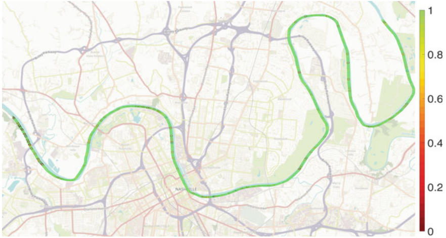
Fig. 4.10 Resulting safety factor distribution for Scenario 1
