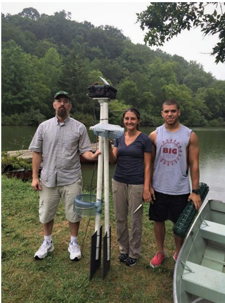
Fig. 18.2 MFC field researchers preparing to install large sediment MFCs (sMFCs) in a pond to enrich naturally occurring electrogens from sediment on the lower graphite anodes and phototrophic, biocathode-associated microbes on the upper carbon cloth cathodes. Left to right: John Pisciotta, Paige Minka, and Jeremy Irving, photo by Nikita Panov
