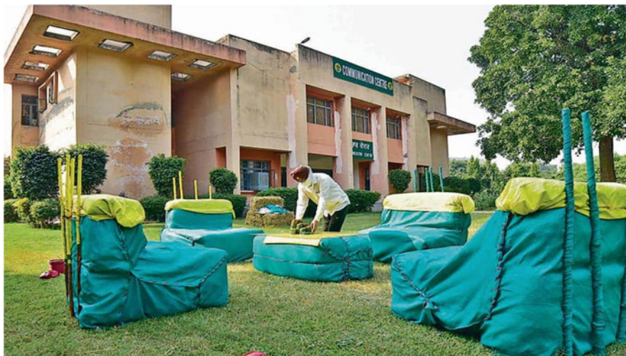
Fig. 1.4 Prepared furniture from paddy stubble as an option to straw burning for reducing C footprints by PAU, Ludhiana (Source: https://www.hindustantimes.com )
