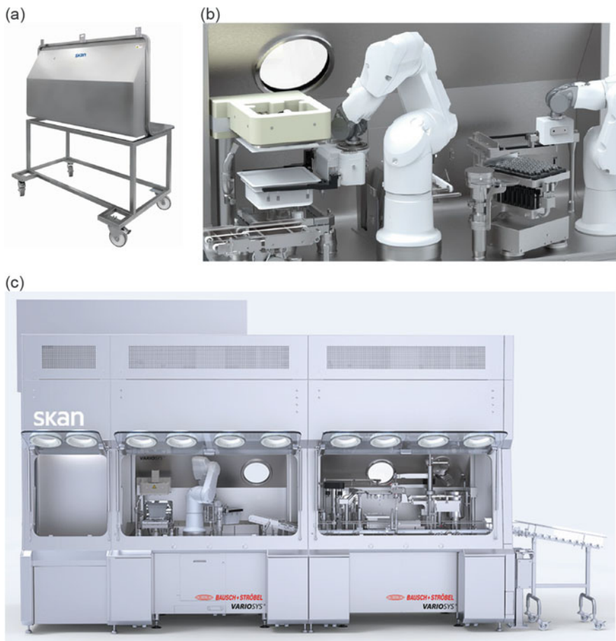
Fig. 12.6 (a) Basic L Flange on webpage. (b) Staubli stericlean robots are mounted on the L-flange of the PSI-L isolator from brochure. (c) VarioSys ® module DDM 9105 for tub opening and denesting (Bausch + Ströbel) fitted in Isolator PSI-L (SKAN) [32]. Reproduced with permission from [33]. Source: SKAN and Bausch + Ströbel Maschinenfabrik Ilshofen GmbH + Co
