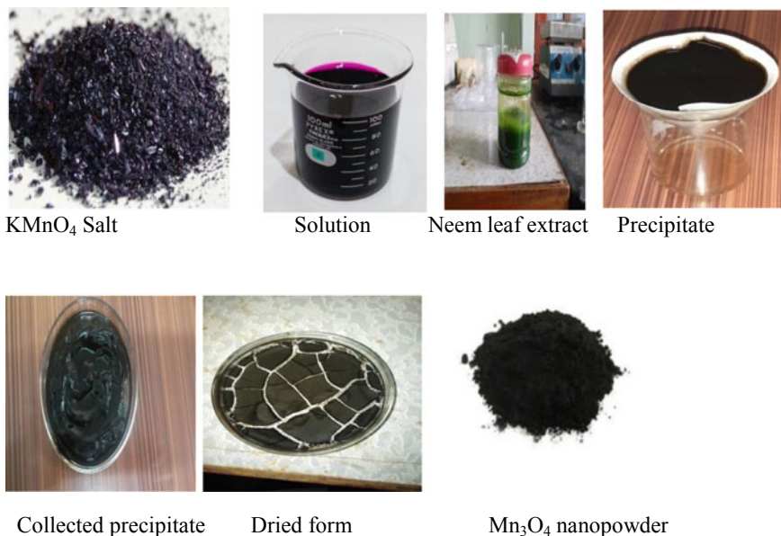
Fig. 3.2 Formation of \text{Mn}_3\text{O}_4 nanoparticles using biosynthesis method
