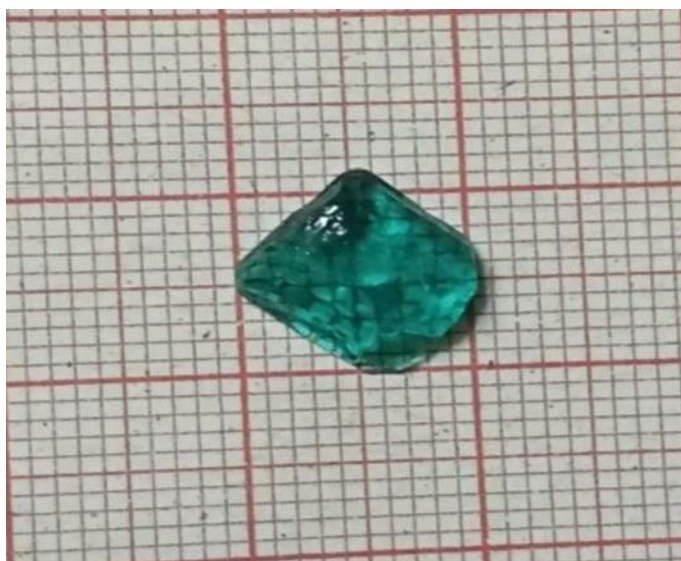
Fig. 14.1 As grown NS:SA single crystal
