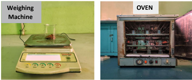
Fig. 21.1 Images of the experimental setup utilized for determining the percentage of soil moisture
