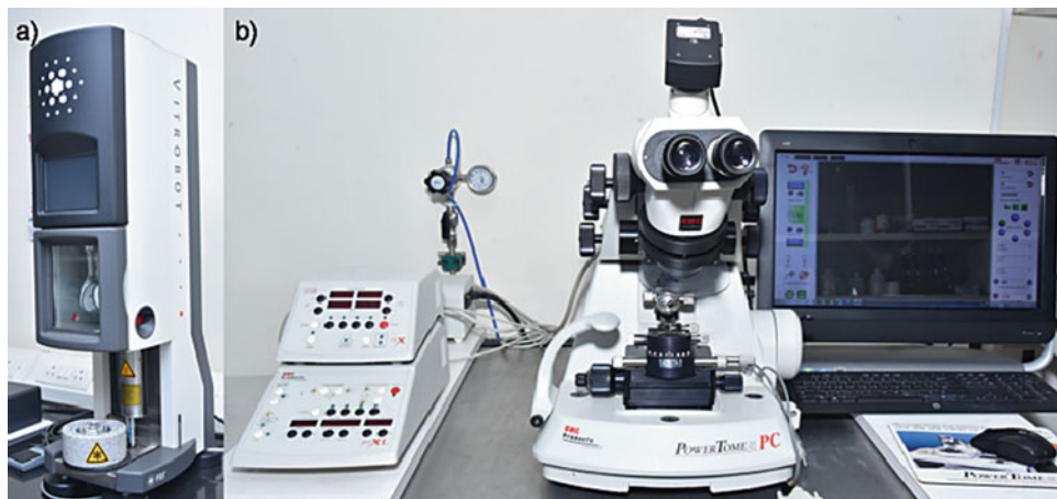
Fig. 9 a Vitrobot for plunge freezing, b Ultramicrotome for sectioning of samples
