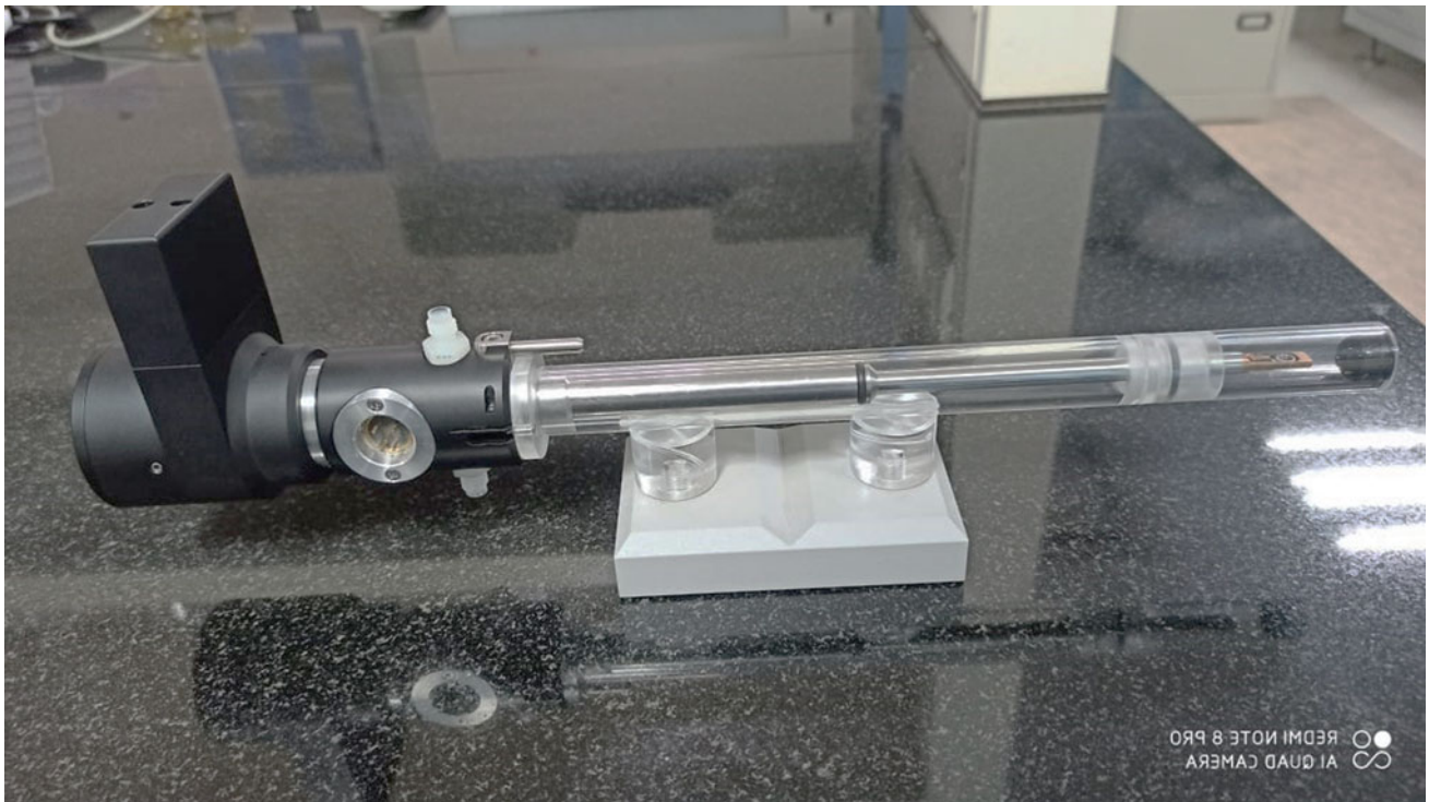
Fig. 3 Photograph of the in-situ heating holder of the Gatan model no. 652 available at advance imaging centre of IIT K
