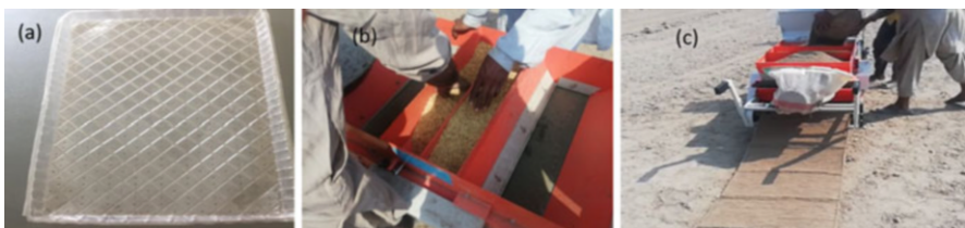
Fig. 3.2 Seedling tray (a), sections of seedling machine (b), and tray filling (c) (Photo by: Zeeshan Haydar)
