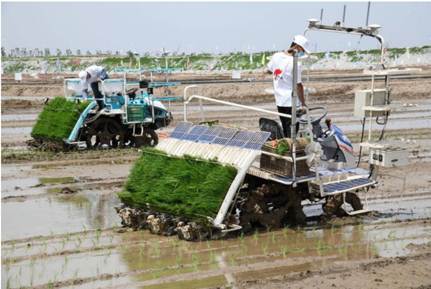
Fig. 3.12 Mechanical transplanting of rice seedlings by transplanter in China (Photo by: Dr. Feng Ling Yang; Dr. Muhammad Ali Raza)
