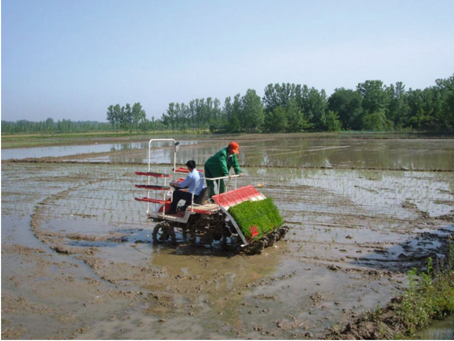
Fig. 3.11 Mechanical transplanting of rice seedlings by transplanter in China (Photo by: Dr. Feng Ling Yang; Dr. Muhammad Ali Raza)
