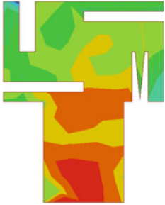
Fig. 10 Current distribution of the proposed antenna
