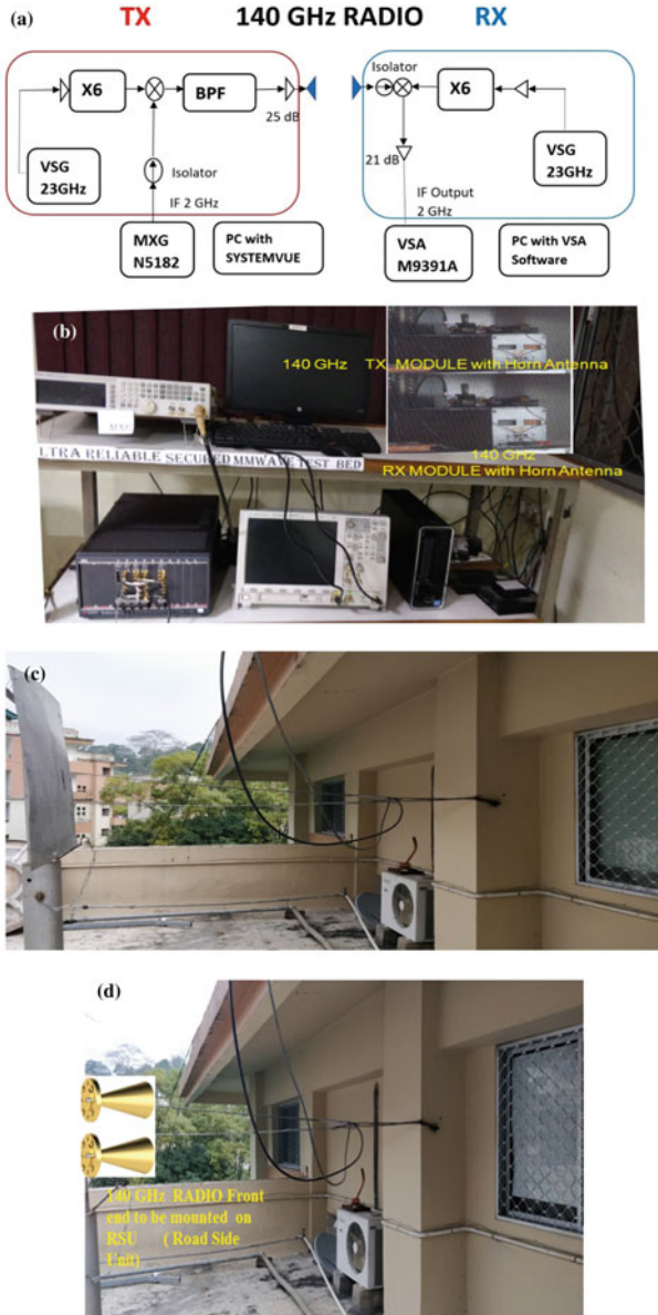
Fig. 4 a Generic Block Diagram of 140 GHz Test Bed to be used as ‘RADAR or 6G Communicator’. b Indoor Unit (IDU) of the Test Bed with 140 GHz TRANCEIVER EMULATING ‘GREEN VEHICLE with 6G RADAR’ on road of Fig. 2. c Outdoor Unit 1 (ODU_1) of the Test Bed with a FLAT Metal Plate EMULATING ‘RED VEHICLE’ on road of Fig. 2. d Outdoor Unit 2 (ODU_2) of the Test Bed with another 140 GHz Radio EMULATING ‘RSU ... Road Side Unit’ on road of Fig. 2
