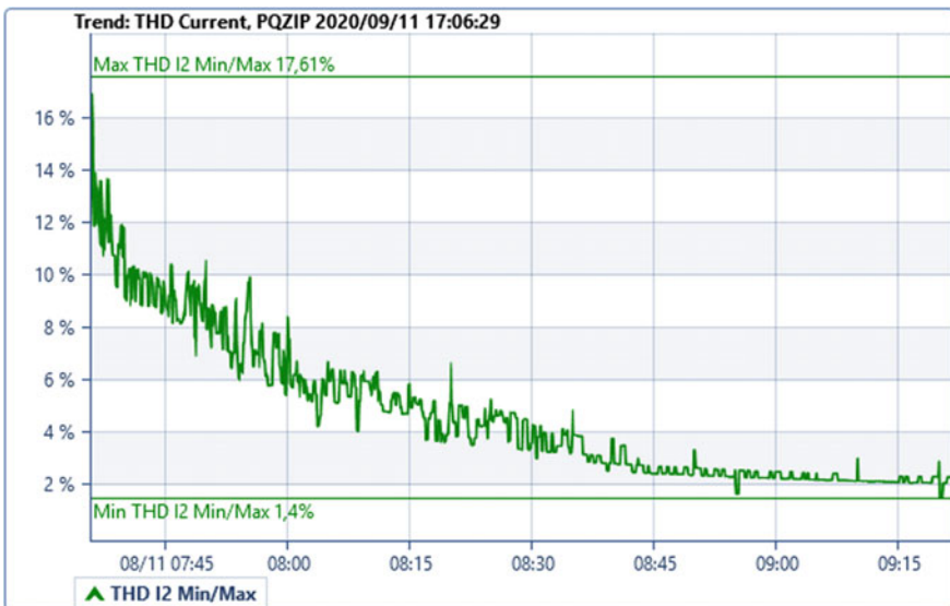
Fig. 10 Sharp decay of current THD during increased solar irradiation
