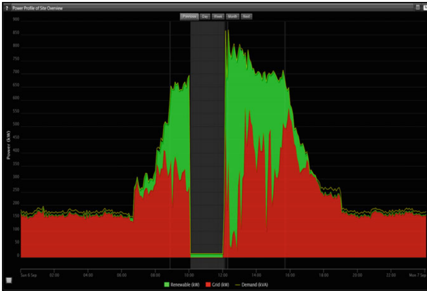
Fig. 5 Loss in PV production during 2 h' load shedding
