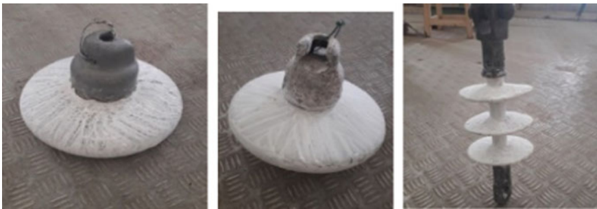
Fig. 3 Coastal polluted ceramic and non-ceramic insulators
