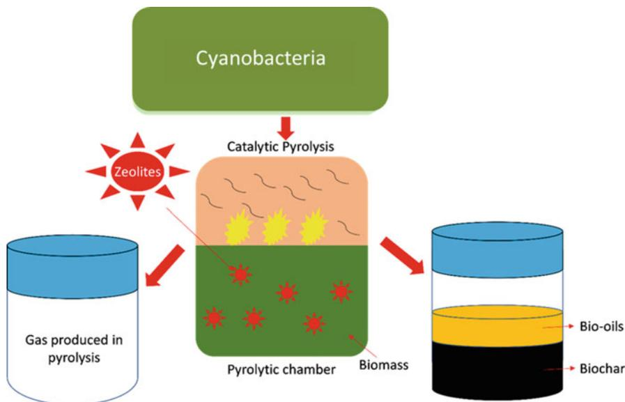
**Fig. 19.3** Schematic representation of cyanobacterial bio-oil production
