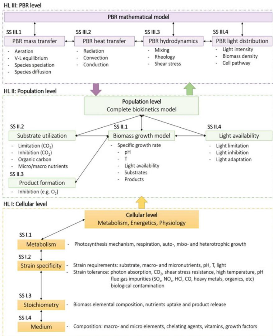
**Fig. 18.1** Scheme of complex PBR model based on System Analysis Theory (HL—hierarchical levels and SS—subsystems). Adapted from Kroumov et al. (2016)
