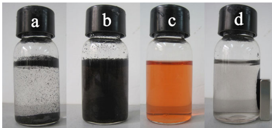
Fig. 18 Optical photographs: a GMCNTs existed in the solution, b CS-m-GMCNTs is dispersed in solution, c solution of the CR dye, d separation of the CS-m-GMCNTs adsorbents from the treated solution of the CR dye by a bar magnet [49, 64]. (To take permission from the Journal of Appl Surf Sci for the https://doi.org/10.1016/j.apsusc.2013.09.003 )
