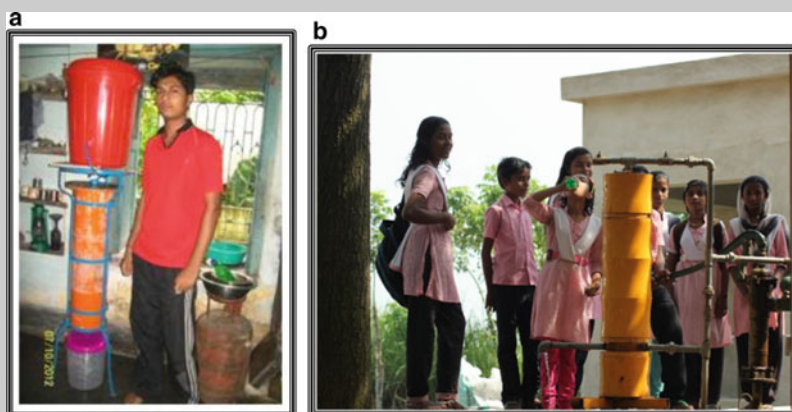
Fig. 9.6 a Laterite based arsenic domestic filters. b Community-scale filter of 500 L/day installed in a primary school in Kashinathpur in Rajarhat, near Kolkata
